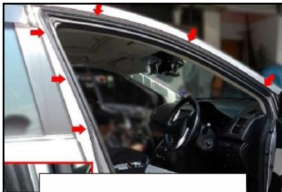
1. Locate the door frame rubber seal
