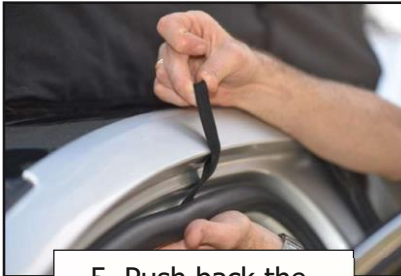
5. Push back the rubber seal to secure the hook in place
