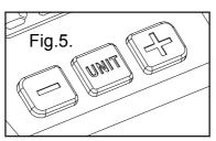
The target pressure level can be changed during inflation process. Press + or - buttons to new desired PSI level.
